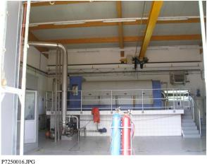
figure 3: chamber press filter (left) and decanter-centrifuge (right)
