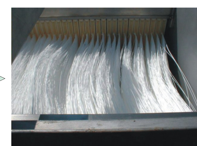
Close look at the polyethylene hollow fibre membranes (0.4µm).
