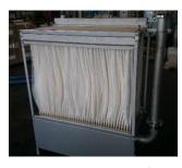
The biological treatment takes place in the MBR tank. Due to the membrane, all biomass in the form of activated sludge is held back and therefore, the sludge age can be freely chosen. Aera-
